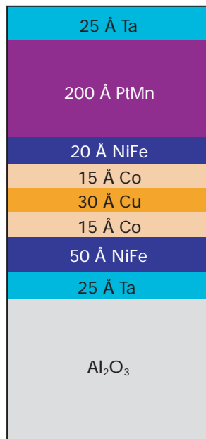
Figure 3 Schematic of a typical spin valve GMR structure found in advanced read sensor devices
