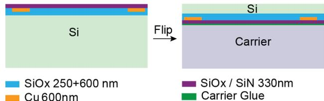
**Figure 7:** Cross section of test wafers with embedded damascene Cu targets. Wafers are inverted, glued to a carrier, and then the silicon is thinned and polished.
