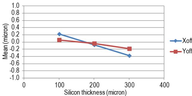
**Figure 13:** Plot of mean versus silicon thickness for LEXT microscope measurement.
