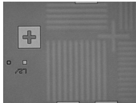
**Figure 11:** View from off-axis camera of resist feature (left cross in box) in focus and embedded metal mark under 200  $\mu\text{m}$  thick silicon which is out of focus. Focus offset is needed to get the embedded mark in proper focus for measurement. Note that the large offset between marks and the non-symmetric nature of the embedded mark prevented reliable TIS measurement from this structure.
