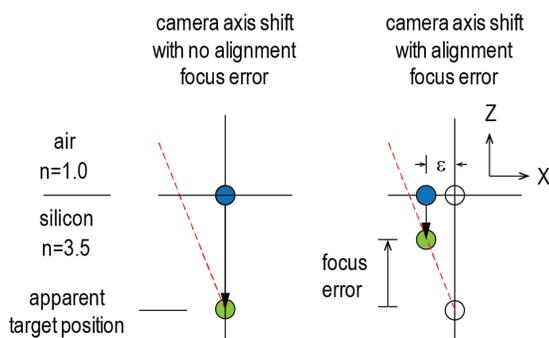
**Figure 3:** Tilt of the alignment system can create a lateral error ( $\epsilon$ ) in captured position if there is an alignment focus error. Focus error will cause the perceived image position to shift along the axis of the alignment system shown as a dotted line. Arrow shows the Z shift translation from the surface position to the corresponding alignment target position.
