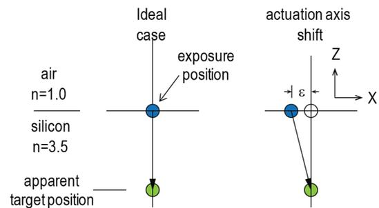
**Figure 4:** Diagram showing the effect on Z-axis tilt on overlay. A Z-axis tilt shifts the target during the Z-axis move from the surface position to the corresponding alignment target position.
