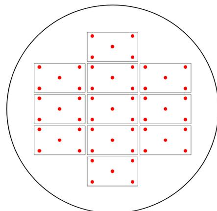
**Figure 8:** Metrology sampling plan on 200 mm wafer. Dots in the wafer map denote measurement locations.
