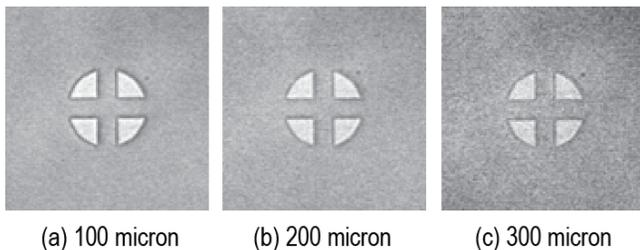
**Figure 10:** Images of DSA targets through three thicknesses of Si.
