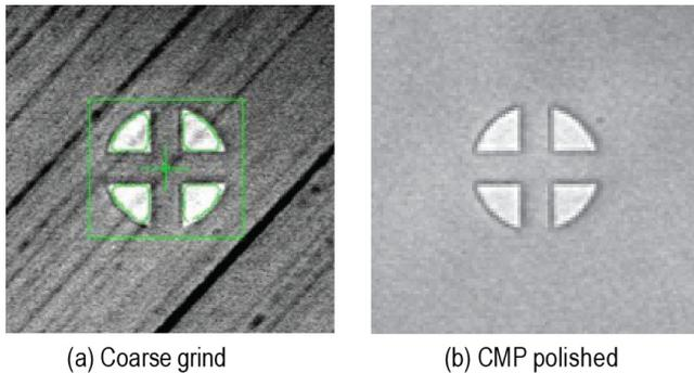
**Figure 9:** DSA camera view of (a) wafer after coarse grinding, (b) wafer after grinding and CMP. The wafer is 100  $\mu\text{m}$  thick silicon.
