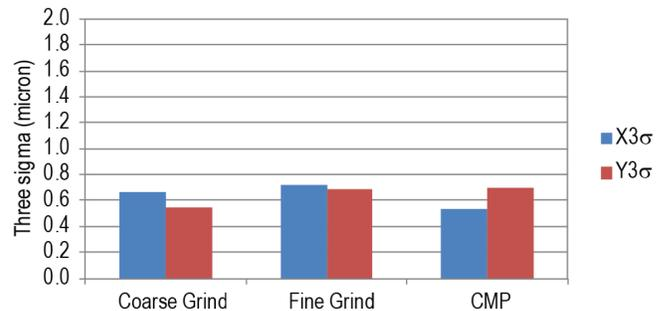
**Figure 16:** Plot of 3-sigma versus polishing technique for 200  $\mu\text{m}$  thick silicon.
