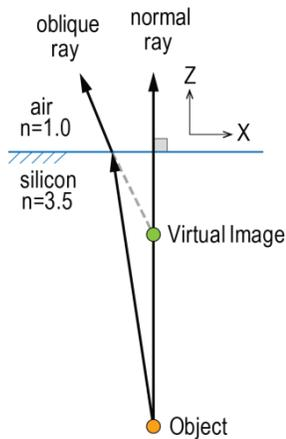
**Figure 2:** Ray trace of the principal ray shows that the apparent target position viewed from the air side appears at different Z position, but has the same XY position as the actual target position.
