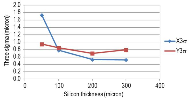
**Figure 15:** Plot of three sigma versus silicon thickness for back-to-front side measurement. Increased variation in X for the 50  $\mu\text{m}$  thick silicon is due to a larger scaling of the wafer pattern, suspected to be caused by distortion of the thin silicon film during the bonding process.
