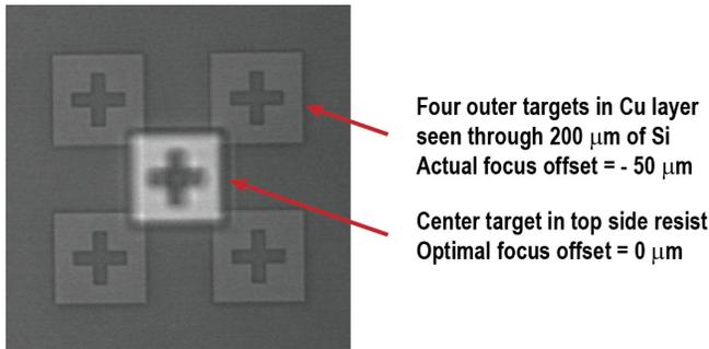
**Figure 5:** The original SSM measurement clover leaf target expects all five sub targets in the same focal plane. This approach does not work for DSA applications: top side and embedded targets are in different focal planes.
