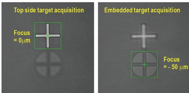
**Figure 6:** New Stepper Self Metrology for DSA changes focus between acquisition of top side and embedded targets. The embedded target is 200 μm into the Si. Note that light refraction at the air/silicon interface makes the virtual image appear higher in Z (-50 μm) than the actual object position (-200 μm).
