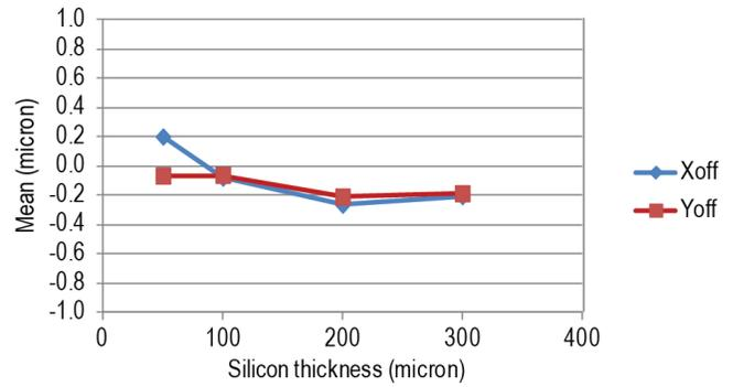
**Figure 14:** Plot of mean versus silicon thickness for back-to-front side measurement.
