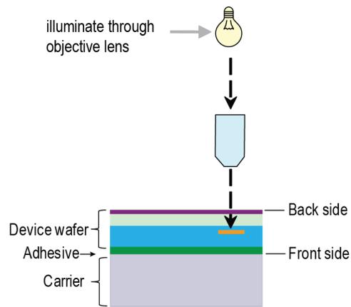
**Figure 1:** Off axis alignment configuration with infrared illumination and imaging from above the wafer. This configuration is the most flexible, providing access to the entire wafer for target alignment.
