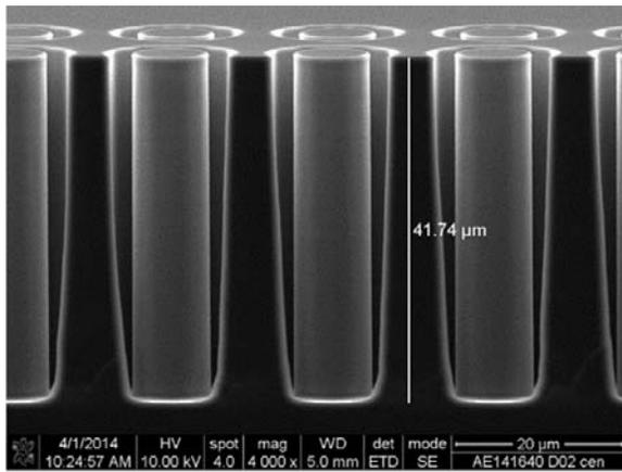
**Figure 5(b):** Cross-section of Donut TSV's etched in Si. The cleave is not perfectly perpendicular to the surface and it appears that the trenches are much narrower at the bottom which is not the case.
