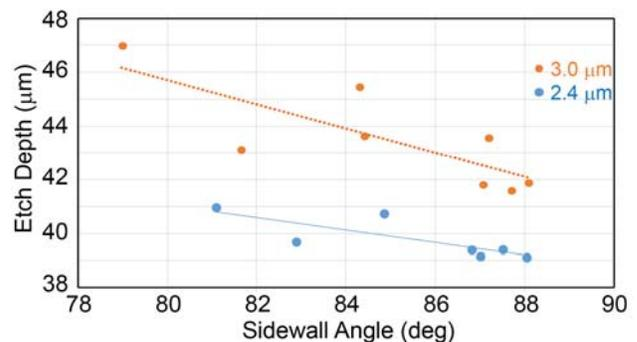
**Figure 12:** Etch depth dependence on CD and sidewall angle.
