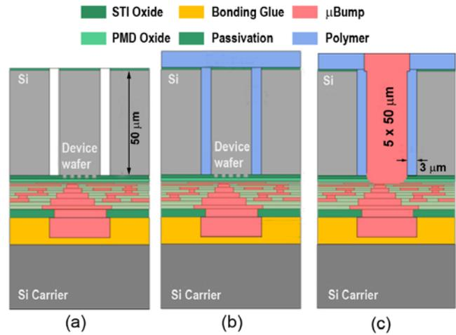
**Figure 1:** Via last module showing (a) Deep-Si trench, (b) filling the trench with polymer material and (c) TSV after complete via last process module [3].
