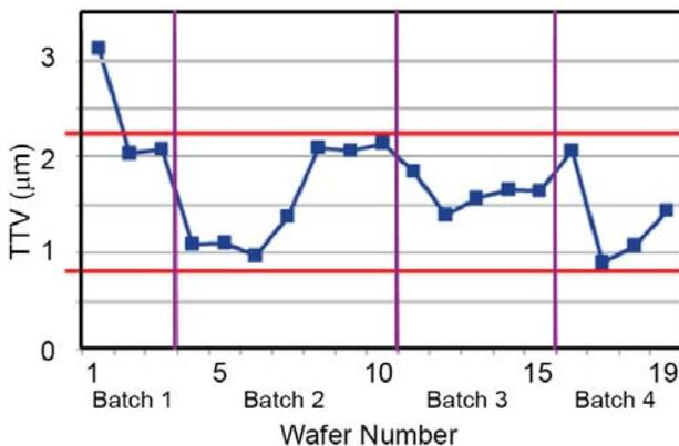
**Figure 14:** Typical TTV of thinned 300mm wafers for four batches. The red lines show the process control limits.
