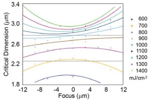
**Figure 7:** Bossung Plot for bottom 2.4μm linear trenches.
