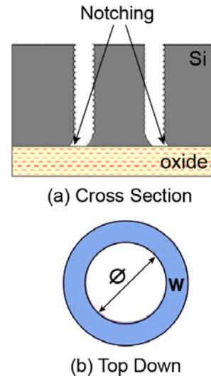
**Figure 2:** (a) Cross sectional drawing of the Si trench stopping on the STI oxide layer. (b) Top down drawing showing typical core width ( $\varnothing$ ) and donut width ( $w$ ).
