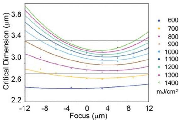
**Figure 6:** Bossung Plot for top CD 2.4μm linear trenches.
