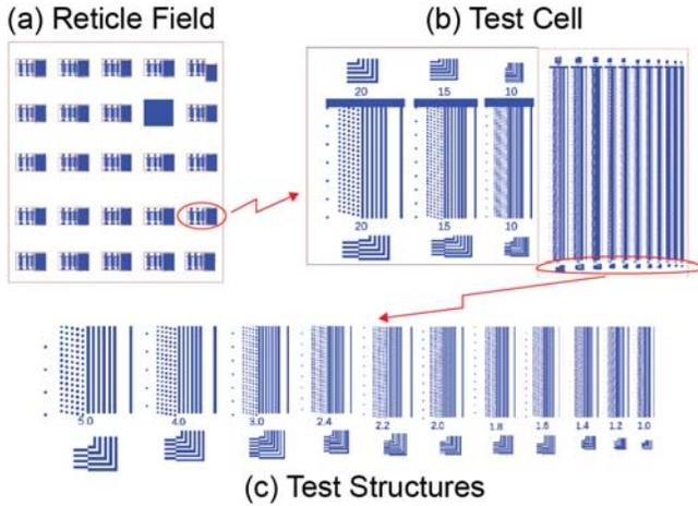
**Figure 3:** Test reticle layout. The reticle field contains an array of test cells which contain the actual test structures.
