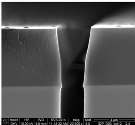
**Figure 10:** Detail view of the top of an etched trench with the photoresist still present.
