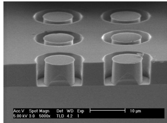
**Figure 5(a):** Cross-section of 2.4 $\mu\text{m}$  Donut TSV's imaged in 7.5 $\mu\text{m}$  thick positive photoresist.
