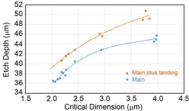
**Figure 13:** Depth after main etch (blue) and main plus landing etch (orange) versus trench width.
