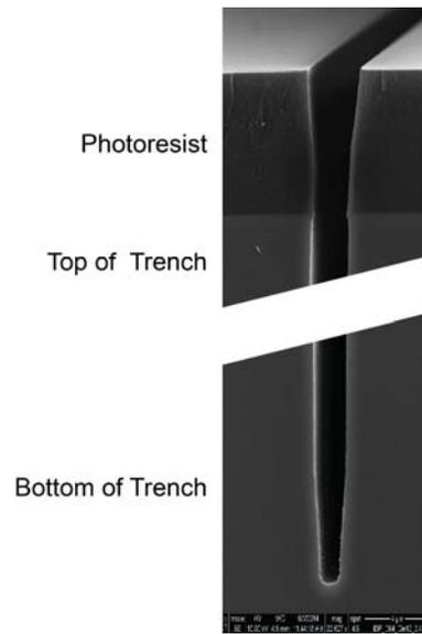
**Figure 11:** Cross-section of trench after main and landing etch. The landing etch at the bottom of the trench shows a smaller CD and more slope than the main etch at the top of the trench.
