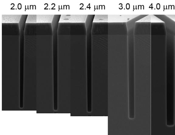
**Figure 9:** Cross-sections of etched trenches. The CD is of is labeled at the top of each trench. Note that the photoresist has not been removed.
