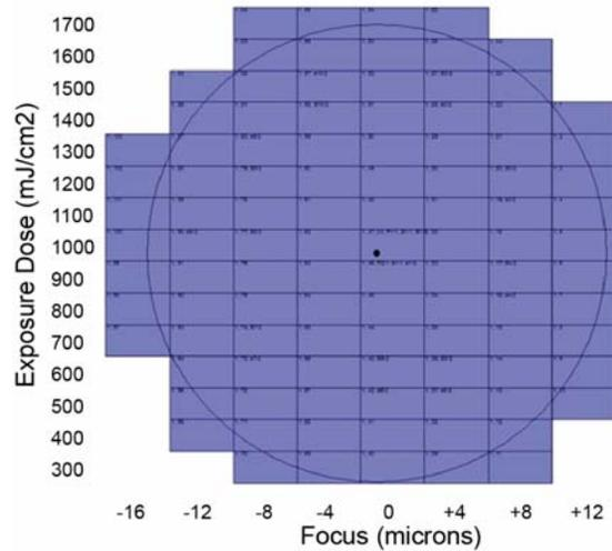
**Figure 4:** Wafer layout for the FEM. An eight by fifteen array was exposed with focus varying in the horizontal axis and exposure dose varying in the vertical axis.
