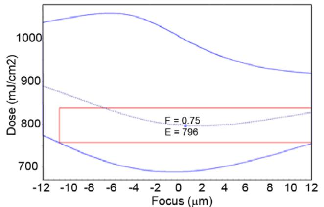
**Figure 8:** Experimental process window for 2.64μm trenches. The blue curves indicate the  $\pm 10\%$  CD limits. The red box is the largest rectangular process window centered at the nominal CD. Sidewall angles are  $\geq 86^\circ$  as determined by cross sectional SEM.
