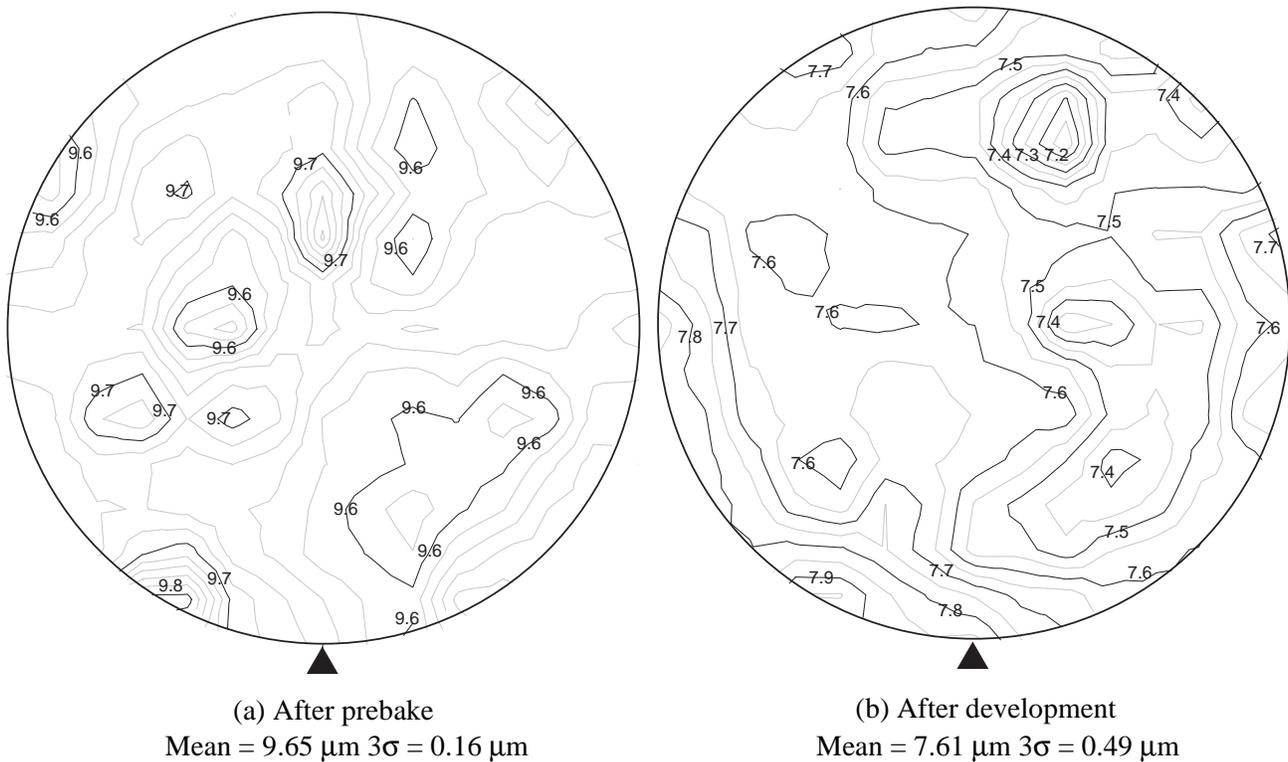
**Figure 4:** Coating uniformity for HD-8001 polyimide on a 300 mm wafer after prebake and after development. The dark contour lines are at 0.1  $\mu\text{m}$  intervals. The three thin spots on the right side of the wafer after development (b) match slots in the wafer cassette used for immersion development.
