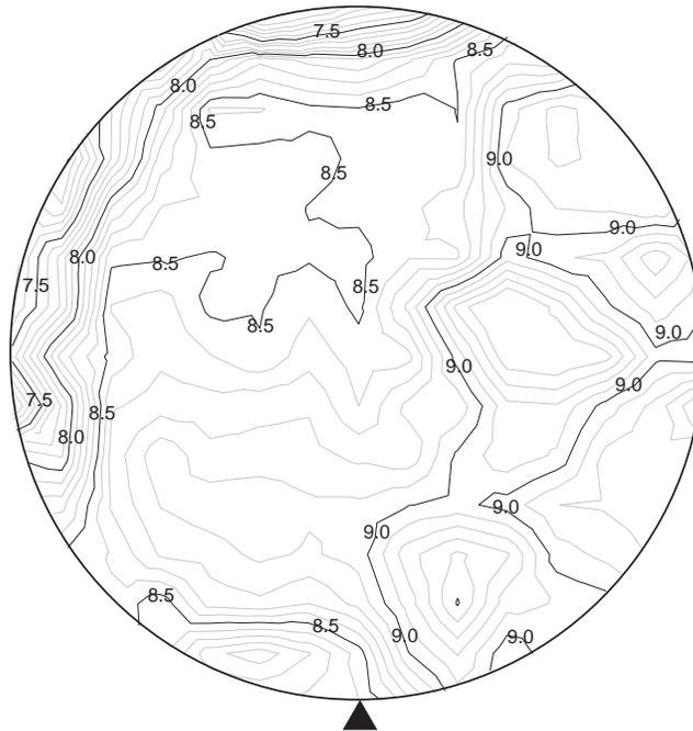
**Figure 8:** CD uniformity for 8  $\mu\text{m}$  spacewidths in HD-8001 polyimide on a 300 mm wafer. The average size is 8.59  $\mu\text{m}$  with  $3\sigma$  of 1.25  $\mu\text{m}$ . The dark contours are at 0.5  $\mu\text{m}$  intervals. The three larger CD spots on the right side of the wafer match the thin polyimide spots seen after development (Figure 4b).
