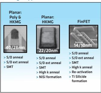
LSA is used for an increasing number of applications as devices scale to smaller dimensions with different materials and architectures
