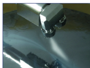
High pressure spray, with point-of-use-heated solvents.
