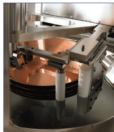
Batch soak complements single wafer spray for stripping dry film resist.
