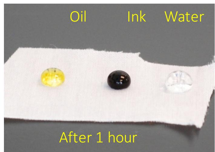
Deposition in Savannah S200 at 80°C, 10 min. exposure
