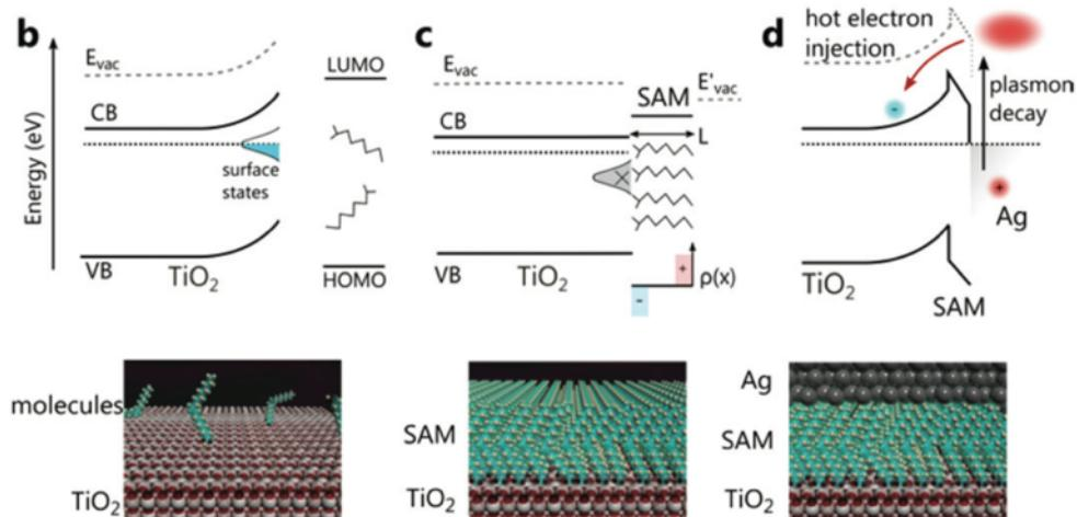
Impact of SAMS length on injection efficiency, photon conversion efficiency and short circuit current
