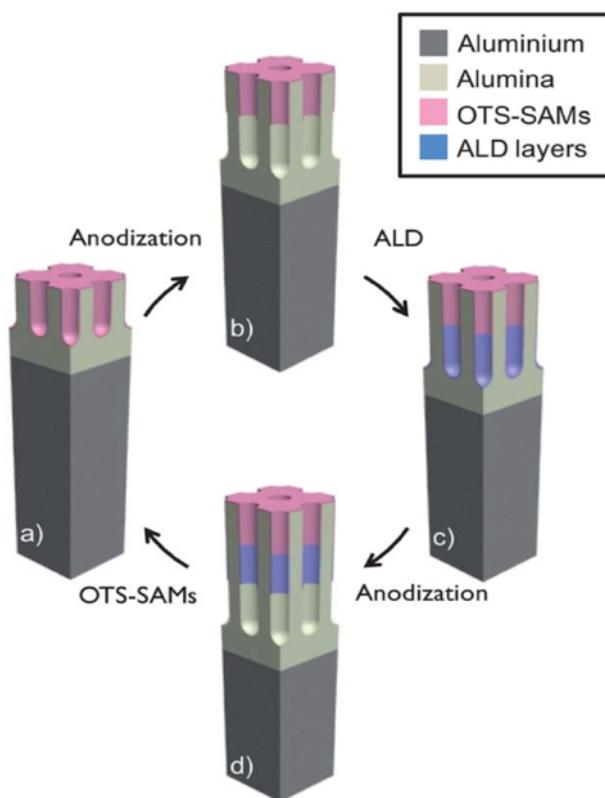
Examples of  $\text{TiO}_2$  /  $\text{ZrO}_2$  segmented nanotubes deposited in AAO nano-template using OTS SAMS
